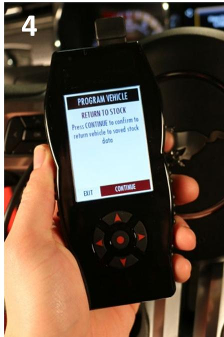
6. Follow device prompts to cycle the key to the ON/OFF position to complete restoring the stock tune:
