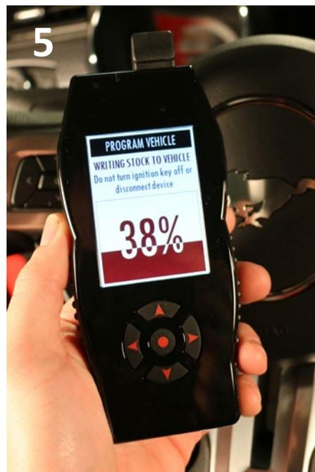
7. Your vehicle will now have the stock tune installed and become "Unmarried" which will allow you to use the device on other vehicles if desired.
